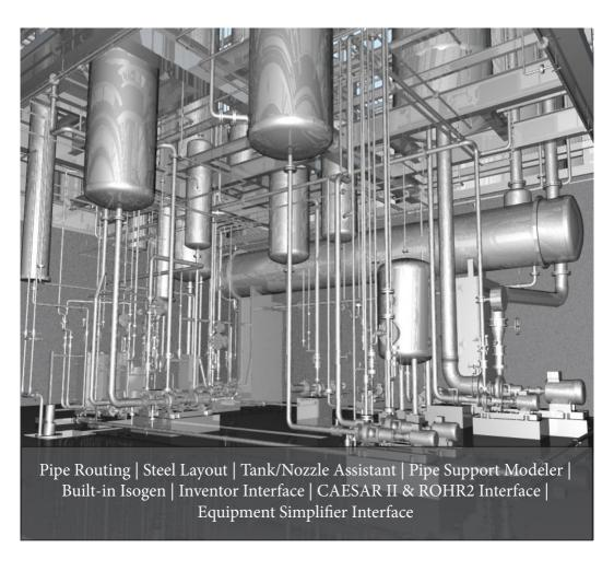
CADISON® 3D-Designer is a complete plant design suite for plant layouts, pipeline routing, equipment modeling, steel layouts, GA & Isometric drawing creation and report generation.
