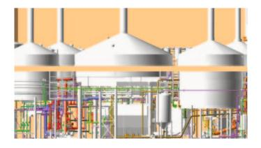
Breweries are particularly suitable for modular design construction and skid, since certain areas need to be redesigned or modernized often. The model shown above was a brewery designed & constructed with DIN 11850 standard. The displayed tanks were developed with the help of integrated 'Tank Assistant' and 'Inventor Interface'. The valves and joists are part of the manufacturer catalogs provided by the customer.
